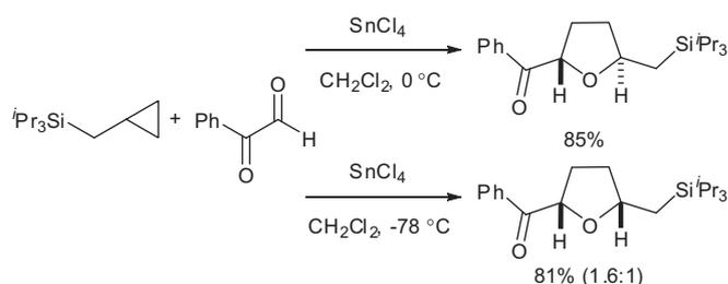
Scheme 1. Synthesis of 2,5-disubstituted tetrahydrofurans.
