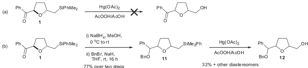
**Scheme 8.** Oxidative removal of the silicon moiety.
