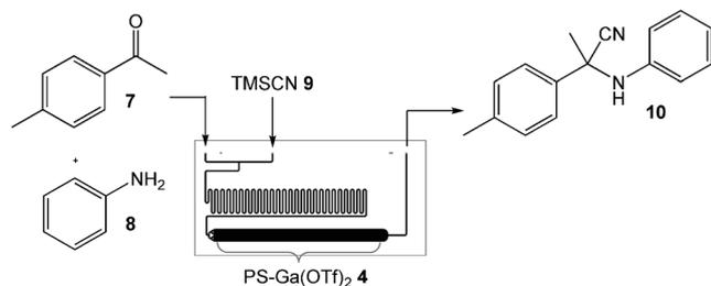
**Figure 2.** The reaction manifold (Labtrix 3026) used to investigate the ketonic Strecker reaction under continuous flow.
