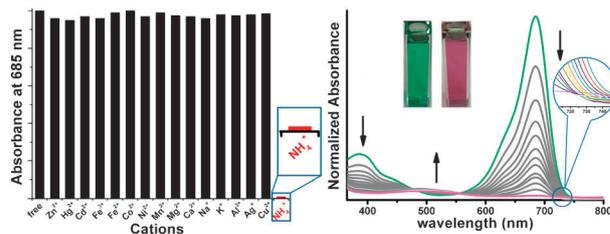
**Fig. 3** Absorption intensity observed at 685 nm upon addition of various metal ions (black) and the  $\text{NH}_4^+$  ion (red) to 10  $\mu\text{M}$  solutions of **3** in THF solution (left). Changes in the absorption spectrum of aza-BODIPY **3** (10  $\mu\text{M}$  in THF) as the ammonium acetate concentration is increased. The inset shows the solution colour before (green) and after (pink) addition of  $\text{NH}_4^+$  (right).
