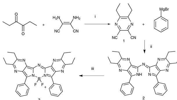
**Scheme 1** Synthetic procedures for aza-BODIPY **3**. (i)  $\text{H}_2\text{O}$ /ethanol (2 : 3), acetic acid, reflux; (ii) dry diethyl ether, RT, 1 h; (iii)  $\text{BF}_3 \cdot \text{OEt}_2$ , triethylamine, dry  $\text{CH}_2\text{Cl}_2$ , reflux.
