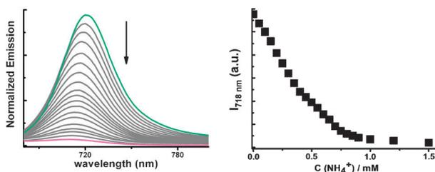
**Fig. 4** Emission spectrum of aza-BODIPY **3** in the presence of increasing  $\text{NH}_4^+$  concentration in THF (left,  $\lambda_{\text{ex}} = 630$  nm). The emission intensity at 718 nm changes as a function of  $\text{NH}_4^+$  concentration (right).
