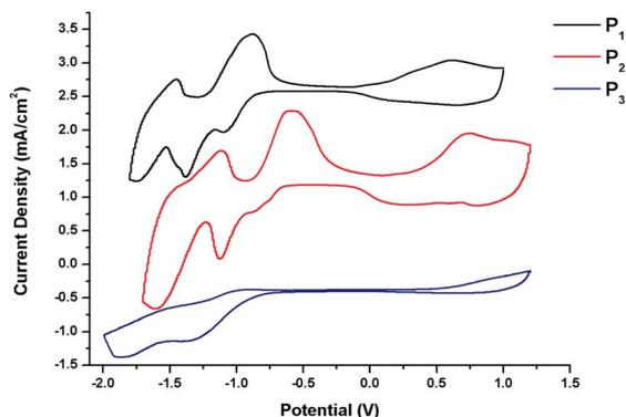
**Fig. 3** Single scan cyclic voltammograms of  $P_1$ ,  $P_2$  and  $P_3$  films using ACN as the solvent and  $0.1 \text{ M TBAPF}_6$  as the supporting electrolyte at a scan rate of  $100 \text{ mV s}^{-1}$  and reduction peaks.
