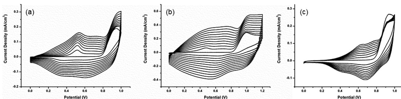
**Fig. 2** Electrochemical polymerizations of (a)  $M_1$  (b)  $M_2$  and (c)  $M_3$  at  $100 \text{ mV s}^{-1}$  in  $0.1 \text{ M TBAPF}_6/\text{CH}_2\text{Cl}_2/\text{ACN}$  on ITO electrodes.
