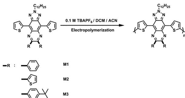
Fig. 1 Electrochemical polymerization of the monomers.
