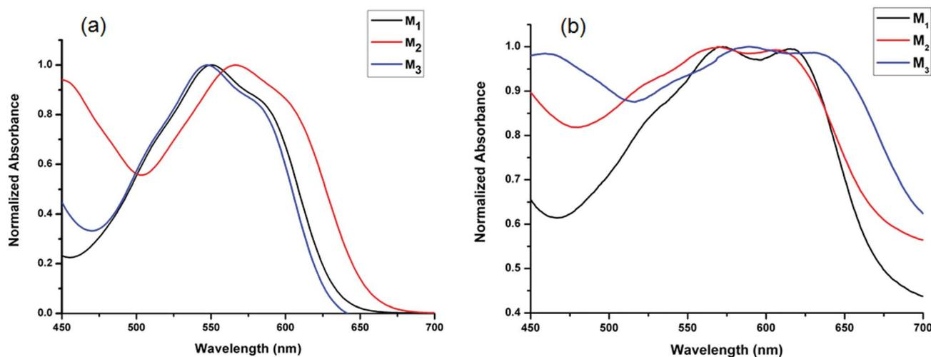
Fig. 5 Absorption spectra of monomers in solution (a) and thin film form (b).
