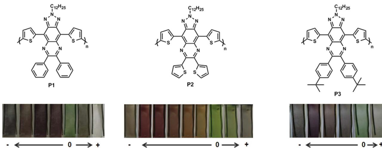
Fig. 6 Structures of the polymers and their colors under different applied potentials.
