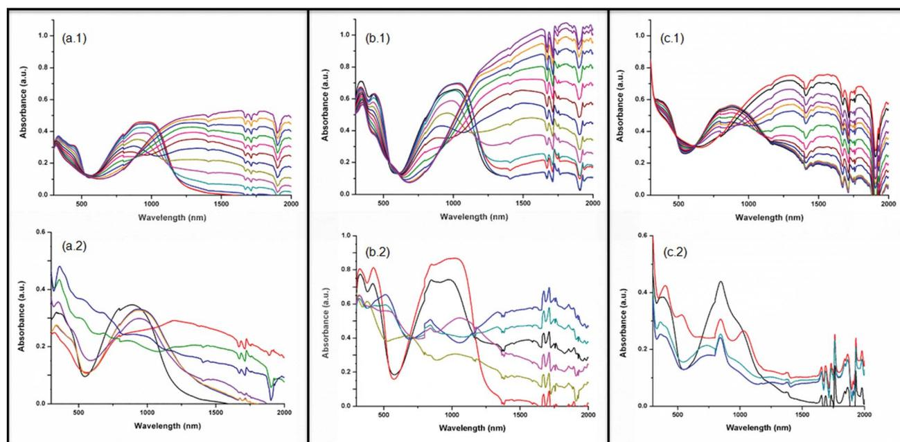
Fig. 4 p-Type doping spectra for P<sub>1</sub> (a.1), P<sub>2</sub> (b.1) and P<sub>3</sub> (c.1) and n-type doping spectra for P<sub>1</sub> (a.2), P<sub>2</sub> (b.2) and P<sub>3</sub> (c.2).
