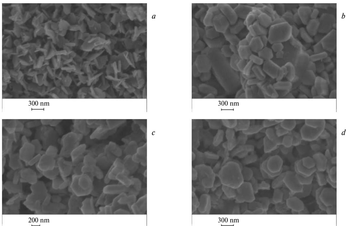
**Fig. 1.** Scanning microphotographs of glass-ceramic samples of compositions **1** (*a, b*) and **2** (*c, d*) synthesized at 800 (*a, c*), 850 (*d*), and 900 °C (*b*). Hexaferrite particles have a hexagonal platelet shape.
