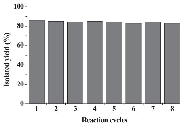
**Fig. 1** Recycling of the MCM-41-2N-RuCl<sub>3</sub> catalyst.
