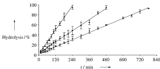
**Figure 1.** Linear plots for the hydrolysis of **9** in HOAc/NaOAc buffer solutions at pH 5.0 (▲), pH 5.5 (■), and pH 6.0 (●). Hydrolyses were performed at 38 °C in the presence of 1-methoxydodecane as an internal standard. Each data point represents the average of three experiments; the bars for each point represent the standard deviation.
