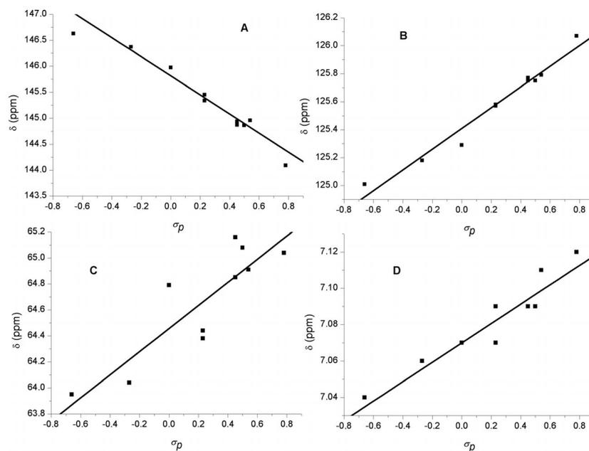
Figure 15. Correlation between NMR chemical shifts (graph A, C-12; graph B, C-15; graph C, C-7; graph D, H-15) and  $\sigma_p$  values in monosubstituted DPNs **5a–j**.
