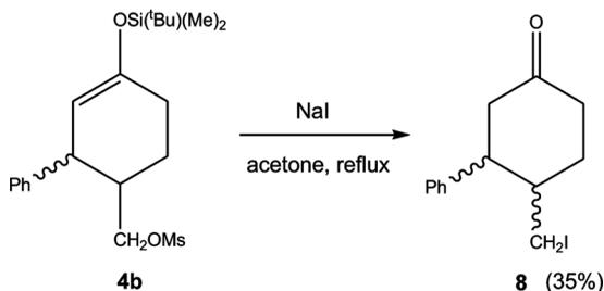
**Scheme 3.** Reaction of exchange between model mesylate **4b** and sodium iodide.
