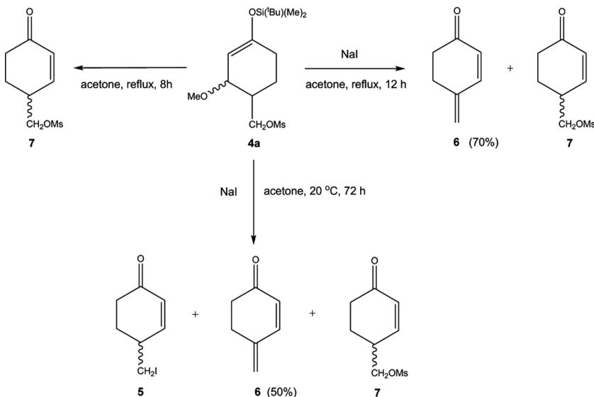
**Scheme 2.** Synthesis of 4-methylenecyclohex-2-enone **6**, mesylate **7**, and iodide **5** from mesylate **4a** under different experimental conditions.
