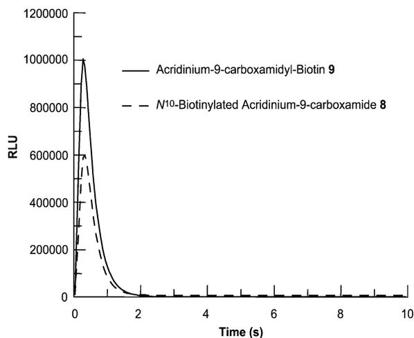
**Figure 2.** Representative luminescence profiles of the *N*-10-tethered and 9-position biotin tracers. Luminescence profiles were obtained by triggering 25  $\mu\text{L}$  aliquots of tracer ( $\sim 0.6$  nM) in 10 mM borate, 2 mM EDTA, 0.1% Tween-20, pH 7.3 using a microplate luminometer (MicroLumat Plus, Perkin-Elmer). Chemiluminescence trigger solution: 200  $\mu\text{L}$  0.18 N NaOH, 0.7%  $\text{H}_2\text{O}_2$ , 1% Triton X-100, 0.05% diethylenetriaminepentacetic acid.
