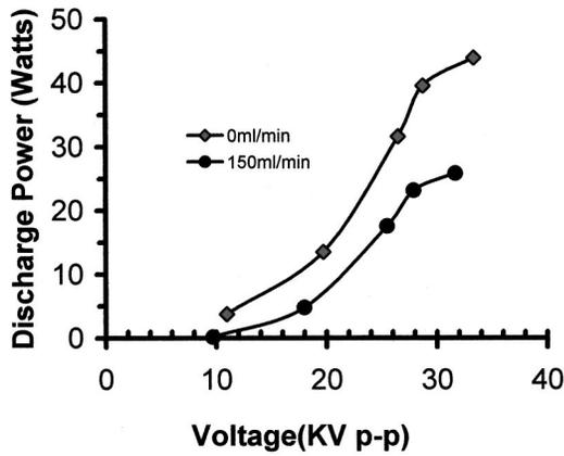
FIG. 2. Discharge power as a function of applied voltage for with and without water flow in the reactor.
