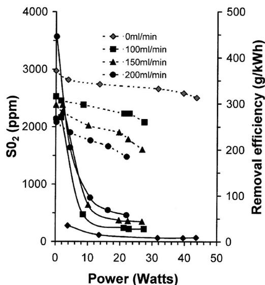
FIG. 3.  $\text{SO}_2$  removal as a function of power. The dashed lines show the  $\text{SO}_2$  concentration for various water flows as a function of discharge power. The solid lines show the energy cost for removal for various water flows as a function of discharge power.
