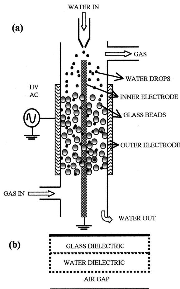
FIG. 1. (a) Schematic of the wet plasma reactor; (b) the equivalent dielectric-barrier discharge representation of a wet plasma reactor.
