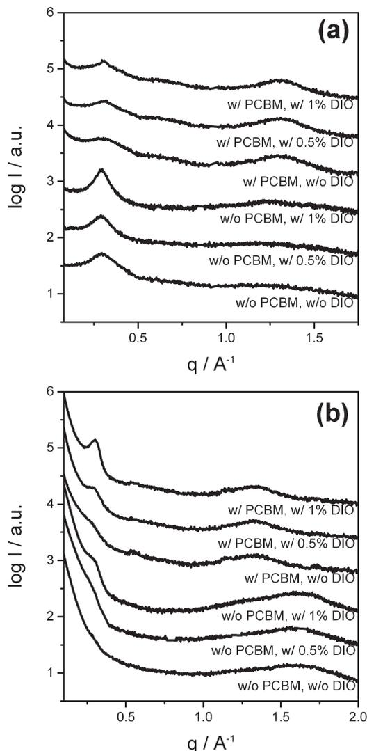
**Figure 3.** In plane (a) and out-of-plane (b) GIXD profiles for the pure films of **PBDTP-DTBT** and the blend of **PBDTP-DTBT**: **PC<sub>71</sub>BM** (1:1.5, w/w) with different amount of DIO.
