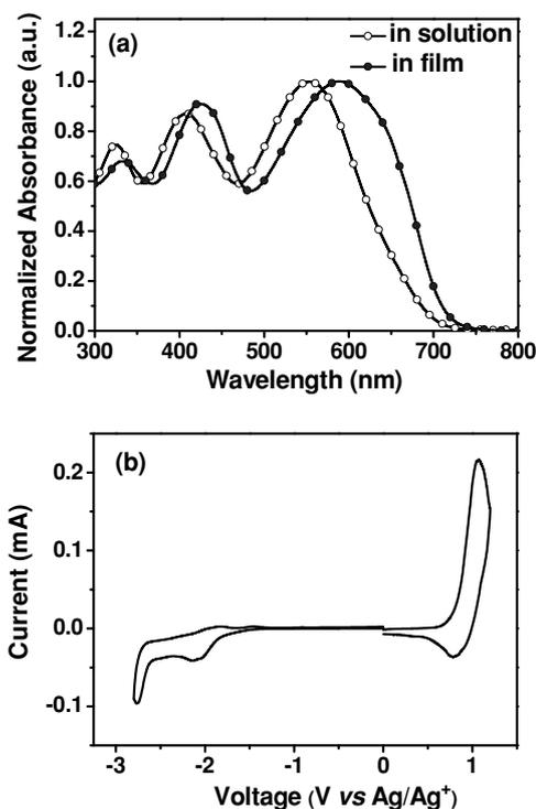
**Figure 1.** (a) The absorption spectra of the polymer in dichlorobenzene and in solid film. (b) Cyclic voltammogram of polymer film on a glassy carbon electrode measured in  $0.1\text{ mol L}^{-1}\text{ Bu}_4\text{NPF}_6$  acetonitrile solution at a scan rate of  $50\text{ mV s}^{-1}$ .
