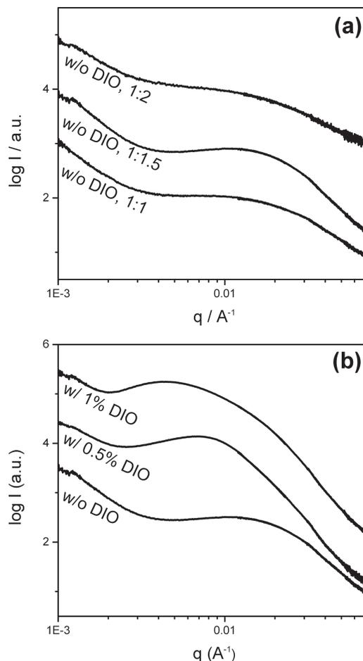
**Figure 4.** RSoXS profiles for (a) **PBDTP-DTBT**: **PC<sub>71</sub>BM** blends processed by o-DCB with different D/A ratios and (b) **PBDTP-DTBT**: **PC<sub>71</sub>BM** (1:1.5, w/w) blends processed by o-DCB, DIO(0.5%)/o-DCB or DIO(1%)/o-DCB, respectively.
