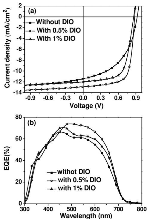
**Figure 2.** (a)  $J$ - $V$  characteristics and (b)  $EQE$  curves of solar cells based on the **PBDTP-DTBT/PC<sub>71</sub>BM** (1:1.5, w/w) blend without and with 0.5% and 1% DIO as additive.
