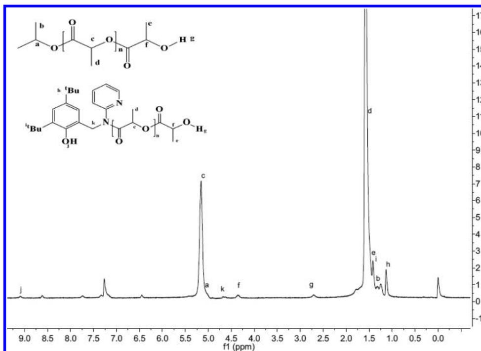
Figure 6.  $^1\text{H}$  NMR spectrum of the oligomer of L-lactide initiated by complex 8 in 70 °C in  $\text{CDCl}_3$ .
