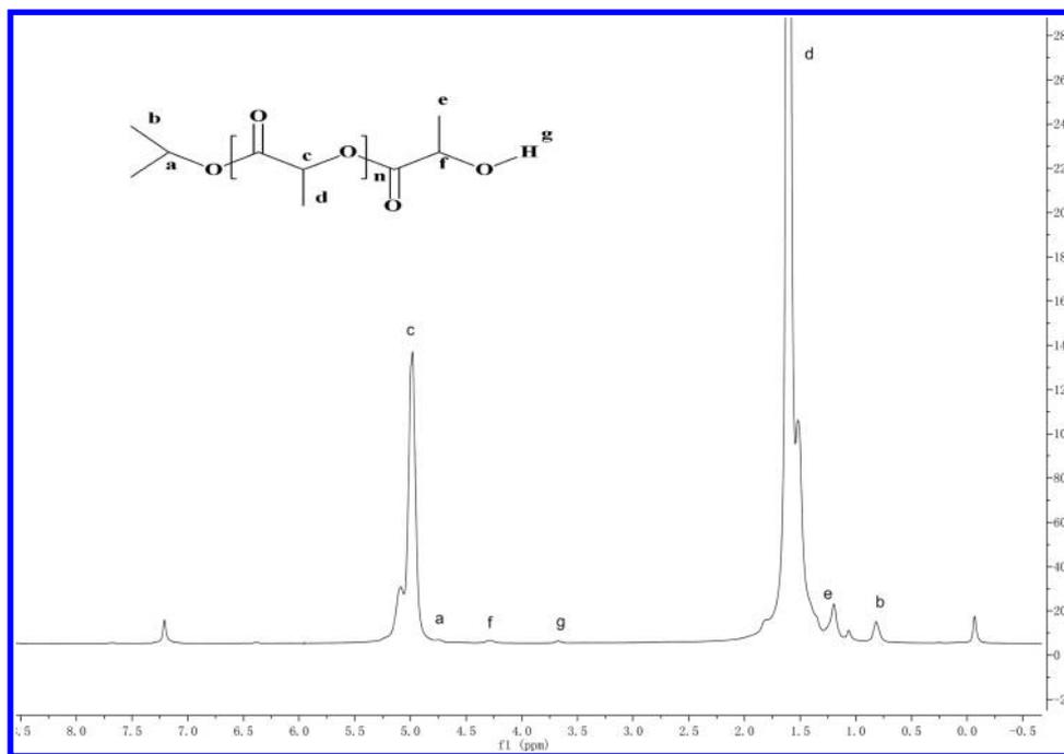
Figure 5.  $^1\text{H}$  NMR spectrum of the oligomer of L-lactide initiated by complex 8 in 25 °C in  $\text{CDCl}_3$ .
