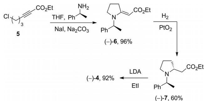
Scheme 2. Synthesis of (*R*)-ethyl 2-[(*R*)-1-[(*S*)-1-phenylethyl]pyrrolidin-2-yl]butanoate (**4**).
