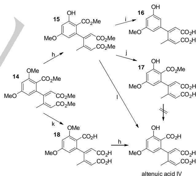
**Scheme 5.** Liberation of altenuic acid IV. Reagents and conditions: (h) BBr<sub>3</sub>, CH<sub>2</sub>Cl<sub>2</sub>, -78 °C → rt, 75 min (**15**: 82%, **AA IV**: 33%); (i) KOH, MeOH, 50 °C, 18 h, then 90 °C, 24 h (52%); (j) NaOH, MeOH, 50 °C, 18 h, then 90 °C, 24 h (quant.); (k) NaOH, MeOH, 50 °C, 24 h (86%); (l) 5M NaOH, 55 °C, 15 h (92%).
