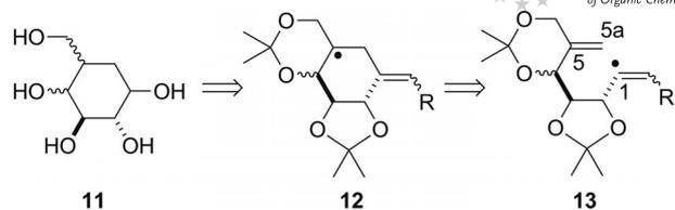
Scheme 2. Retrosynthesis of the carbahexopyranoses **11** by 6-*endo-trig* radical cyclization of the carbohydrate-derived vinyl radicals **13**.
