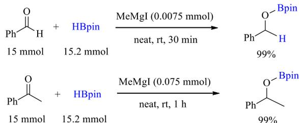
**Scheme 2.** Large-Scale Reaction of Benzaldehyde/Acetophenone with HBpin.
