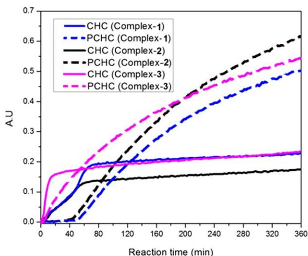
**FIGURE 2** Absorbance versus time profiles of poly(cyclohexene carbonate) (PCHC) and cyclohexene carbonate (CHC) with [ONSO]CrCl complexes (**1–3**). Reaction conditions: [CHO]/catalyst/cocatalyst = 1400/1/2, 3.4 MPa, 80 °C. Dashed and continuous lines represent PCHC and CHC, respectively. [Color figure can be viewed in the online issue, which is available at [wileyonlinelibrary.com](http://wileyonlinelibrary.com).]
