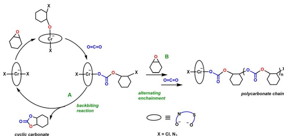
**SCHEME 2** Proposed mechanism for the production of cyclohexene carbonate, Path A and poly(cyclohexene carbonate), Path B. [Color figure can be viewed in the online issue, which is available at [wileyonlinelibrary.com](http://wileyonlinelibrary.com).]
