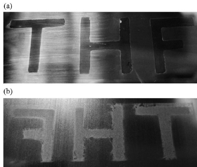
Fig. 8. The photographs of (a) cathode and (b) anode after the pattern electroplating using gel electrolyte. The gel electrolyte contained 0.5 \text{ mol/dm}^3 \text{ Ni(ClO}_4)_2 \cdot 6\text{H}_2\text{O} , 0.5 \text{ mol/dm}^3 \text{ LiCl} . The cathode substrate was copper. The current density was -1 \text{ mA/cm}^2 . The average thickness of gel electrolyte was about 0.55 mm. The plating time was set at 2000 s.
