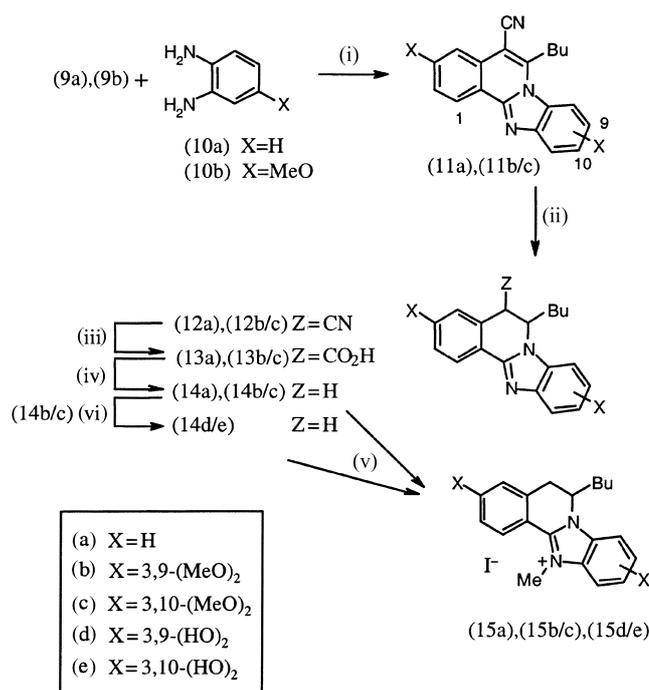
**Scheme 4.** Reagents and conditions: (i) NEt<sub>3</sub>/dioxan/reflux; (ii) NaBH<sub>4</sub>/EtOH; (iii) 57% H<sub>2</sub>SO<sub>4</sub>/reflux; (iv) heat 165–180°C; (v) MeI/EtOAc/reflux; (vi) HBr–HOAc/reflux.
