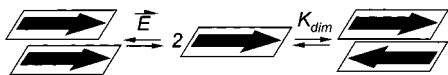
Scheme 4. Model for the Competition between External and Internal Forces in the Electric-Field-Induced Poling Process of Dipolar Dyes in Amorphous Composite Materials
