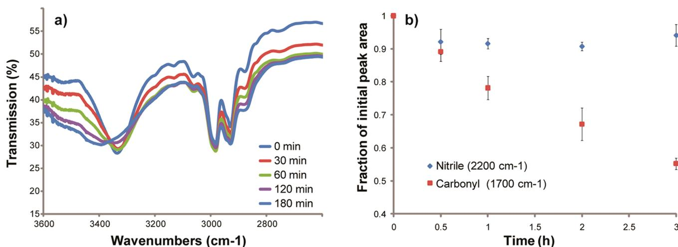
**Figure 2.** (a) Selected IR spectra of films and (b) relative peak ratios of carbonyl and nitrile stretches of precursor **13b** (as a 200 mM solution in a mixture of 11% poly(methacrylonitrile) in nitromethane) as a function of curing times at 160 °C.
