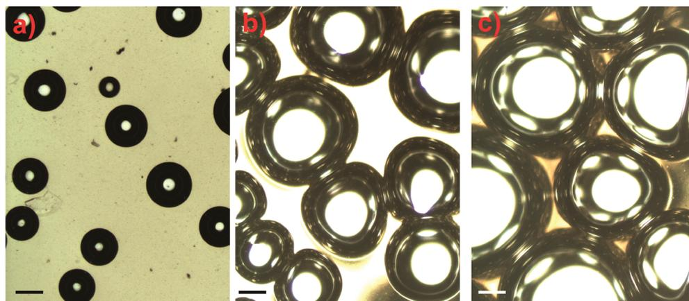
Figure 5. Comparison of  $\text{CO}_2$  bubbles produced in cured resins of epoxy **23**, cured fully at different temperatures: (a)  $160\text{ }^\circ\text{C}$  for 1 h; (b)  $180\text{ }^\circ\text{C}$  for 30 min; (c)  $200\text{ }^\circ\text{C}$  for 15 min. Scale bar is  $200\text{ }\mu\text{m}$ .
