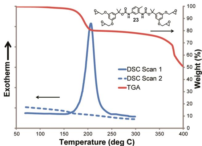
**Figure 3.** Combined DSC and TGA traces for monomer **23**.
