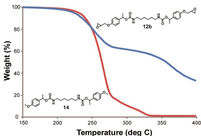
Figure 1. Comparison of TGA traces for monomer 12b (blue) and control 14 (red).
