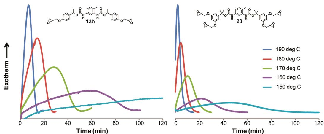
Figure 4. DSC isothermal comparison of monomers **13b** and **23**.
