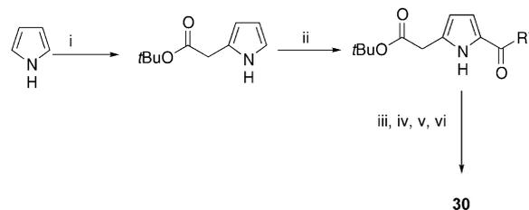
**Scheme 4.** (i)  $\text{BrCH}_2\text{CO}_2t\text{-Bu}$ ,  $\text{EtMgBr}$ ,  $\text{THF}$ ,  $-10^\circ\text{C}$  to rt; (ii)  $R^4\text{C}(\text{Cl})=\text{NMe}_2^+\text{Cl}^-$ ,  $\text{DCM}$ ; (iii) aq  $\text{NaOAc}$ ; (iv)  $\text{TFA}/\text{DCM}$ ; (v)  $(\text{COCl})_2$ , cat  $\text{DMF}$ ,  $\text{DCM}$ ,  $0^\circ\text{C}$ ; (vi) A or B, cat  $\text{DMAP}$ ,  $\text{DCM}$ .
