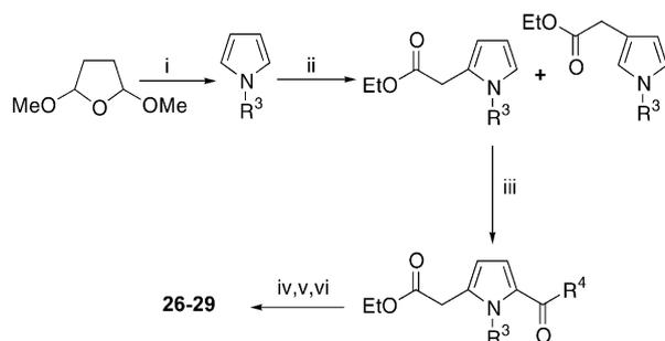
**Scheme 2.** (i)  $R^3\text{NH}_2$ ,  $\text{HOAc}$ , heat; (ii)  $\text{N}_2=\text{CHCO}_2\text{Et}$ ,  $\text{Cu}$  (bronze), heat; (iii)  $R^4\text{COCl}$ , toluene, heat; (iv)  $\text{LiOH}$ ,  $\text{THF}/\text{H}_2\text{O}$ ; (v)  $(\text{COCl})_2$ , cat  $\text{DMF}$ ,  $\text{DCM}$ ,  $0^\circ\text{C}$ ; (vi) A or B, cat  $\text{DMAP}$ ,  $\text{DCM}$ .
