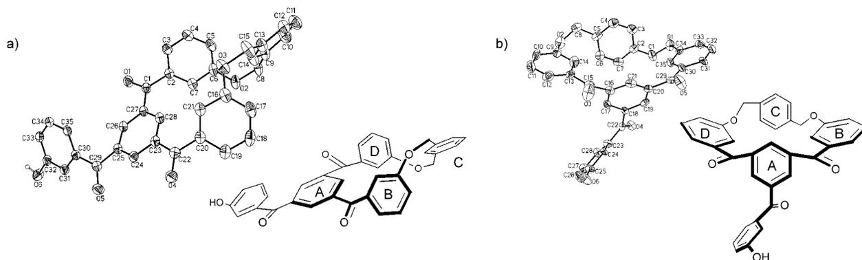
**Figure 2.** (a) Molecular structure (ORTEP) of **8** accompanied by a line drawing representation of the solid-state conformation. (b) The molecular structure (ORTEP) of **9** accompanied by a line drawing representation of the solid-state conformation.
