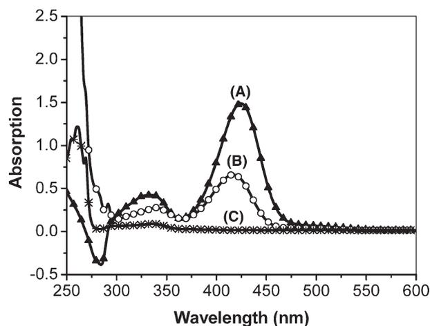
**FIGURE 6** UV-vis spectra of THF solution of (A) CPDADB (0.0125 mg/mL); precipitated PS samples (0.5 mg/mL) (B) **P7** (yellow) and (C) **P7** after the removal of thiocarbonyl end group (white) obtained by heating the THF solution at 60°C for 2 days.
