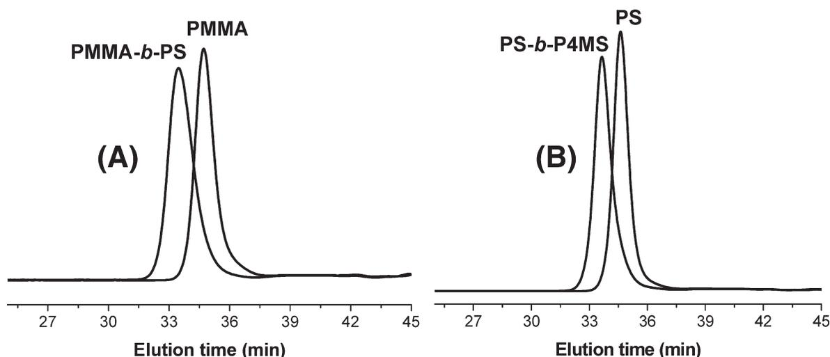
**FIGURE 4** GPC traces of (A) PMMA and PMMA-*b*-PS copolymer and (B) PS and PS-*b*-P4MS copolymer synthesized by respective chain extension reactions.
