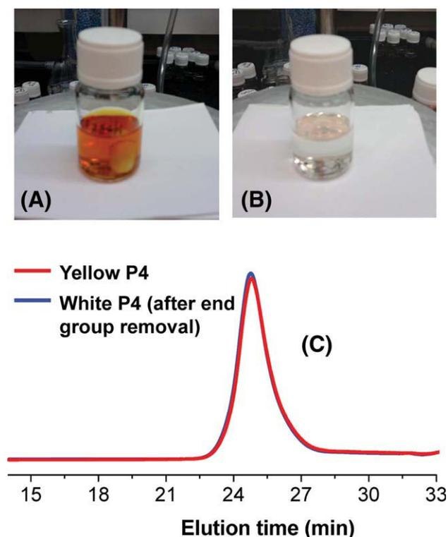
**FIGURE 7** Photograph of relatively low molecular weight PMMA: (A) THF solution of yellow **P4**, (B) the same solution after heating at 60 °C for 1 h in presence of five drops of conc. HCl and (C) overlay GPC chromatograms of yellow **P4** before end group removal (red line) and white PMMA after end group removal (blue line) obtained by the HCl treatment.
