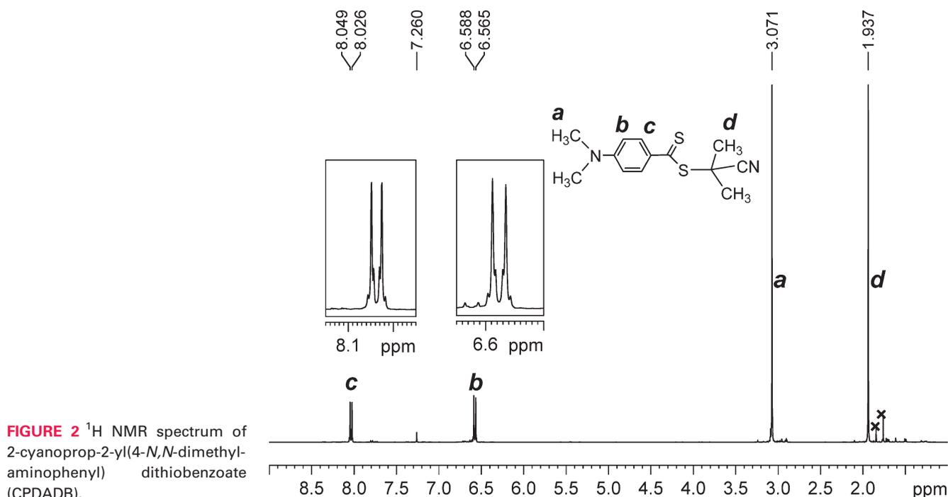
**FIGURE 2** <sup>1</sup>H NMR spectrum of 2-cyanoprop-2-yl(4-*N,N*-dimethylaminophenyl) dithiobenzoate (CPDADB).
