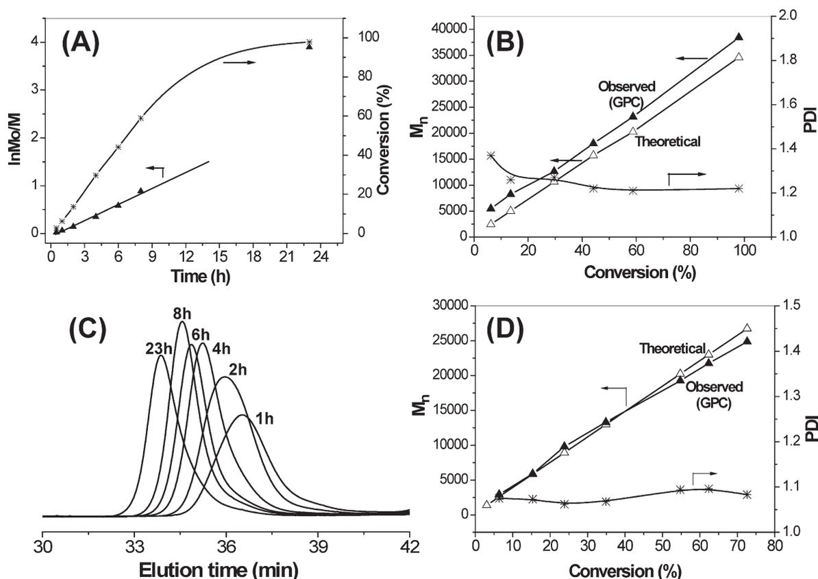
**FIGURE 3** (A) Kinetic plots, (B) evolution of  $M_n$  and PDI with monomer conversion and (C) GPC traces of MMA polymerization using CPDADB; (D) evolution of  $M_n$  and PDI in St polymerization using CPDADB.
