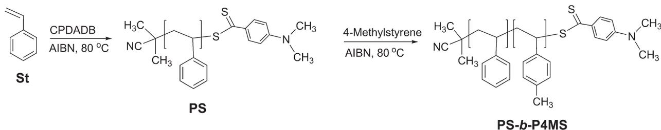
**SCHEME 1** Synthesis of di-block copolymer by chain extension reaction.
