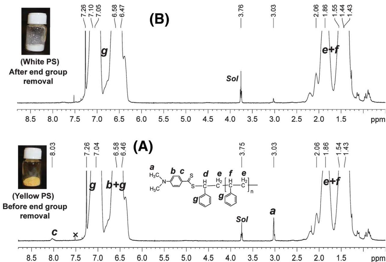
**FIGURE 5** Photograph and <sup>1</sup>H NMR spectra of PS samples (after precipitation from methanol) (A) **P7** (yellow) and (B) **P7** after the removal of thiocarbonyl end group (white) obtained by heating the THF solution at 60°C for 2 days (sol = solvent). [Color figure can be viewed in the online issue, which is available at [wileyonlinelibrary.com](http://wileyonlinelibrary.com).]
