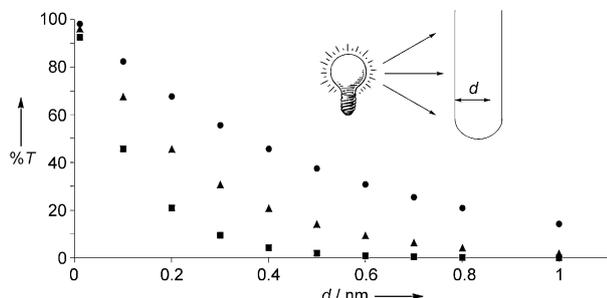
**Figure 1.** The percent transmittance versus distance from the wall ( $d$ ) as calculated from the Beer–Lambert law. ● 0.5 mM  $[\text{Ru}(\text{dmb})_3]^{2+}$ , ▲ 1 mM  $[\text{Ru}(\text{dmb})_3]^{2+}$ , ■ 2 mM  $[\text{Ru}(\text{dmb})_3]^{2+}$ .
