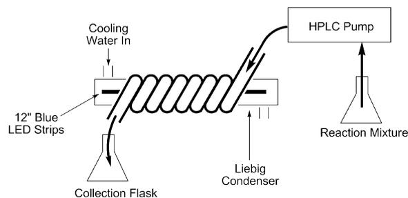
**Figure 2.** Diagram of the designed photoflow reactor.
