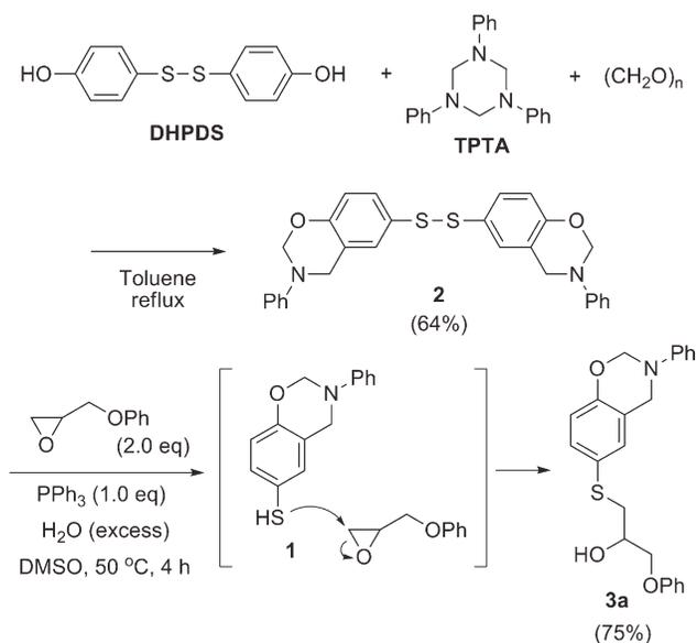
**SCHEME 2** Synthesis and utilization of thiol-functionalized benzoxazine **1**.
