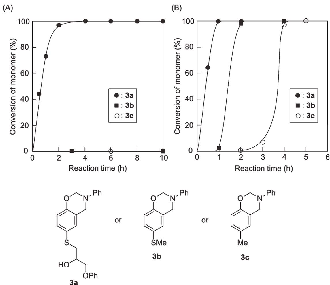
**FIGURE 2** Time-conversion plots for the thermally induced polymerizations of benzoxazines: (A) at 150 °C; (B) at 180 °C.
