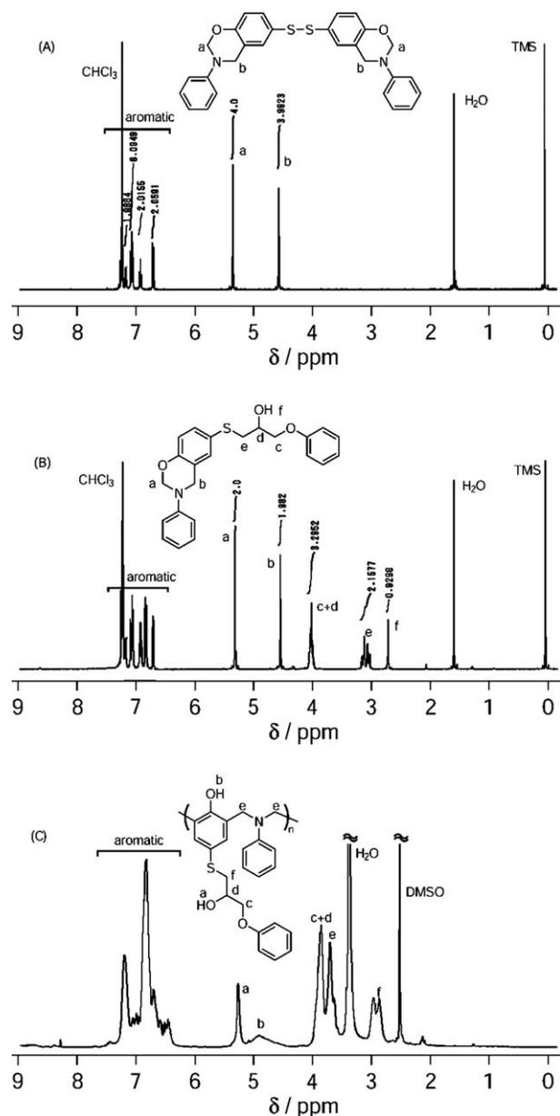
**FIGURE 1**  $^1\text{H}$  NMR spectra of benzoxazines **2** (A), **3a** (B), and polymer **4a** obtained after heating for 2 h at 180 °C (C).
