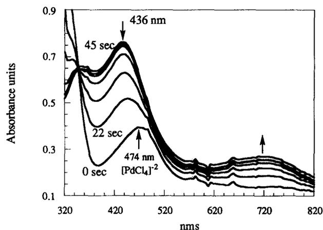
Fig. 1. UV-Vis spectral changes for the first 45 s during the formation of the catalytically active complex from  $3.1 \times 10^{-3}$  M  $[\text{PdCl}_4]^{2-}$ , 800 torr NO, and 0.1 M CuCl in 2 M HCl.
