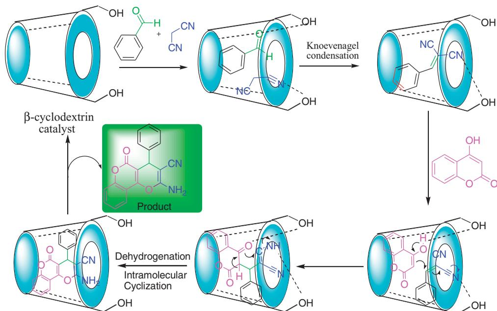
**Scheme 4.** Plausible reaction mechanism for the synthesis of 4H,5H-pyrano[3,2-c][1]benzopyran-5-ones (**4a**).
