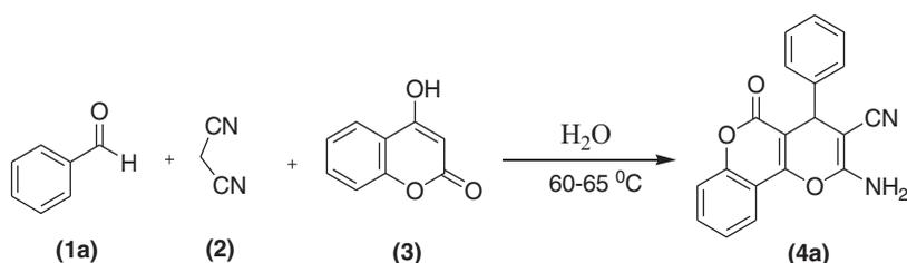
**Scheme 1.** Synthesis of 2-amino-4,5-dihydro-5-oxo-4-phenylpyrano[3,2-c]chromene-3-carbonitrile (**4a**) (model reaction).
