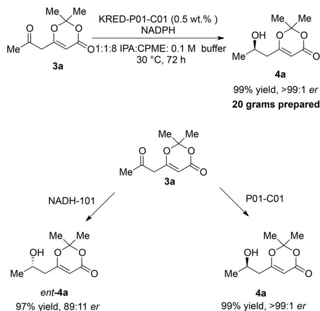
**Figure 5.** Large-scale reduction of  $\beta$ -ketodioxinone and access to both enantiomers of  $\beta$ -hydroxydioxinone **4a**.
