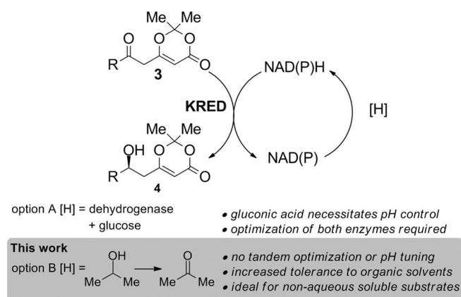
**Figure 3.** Catalytic cycle of ketoreductase enzymes.
