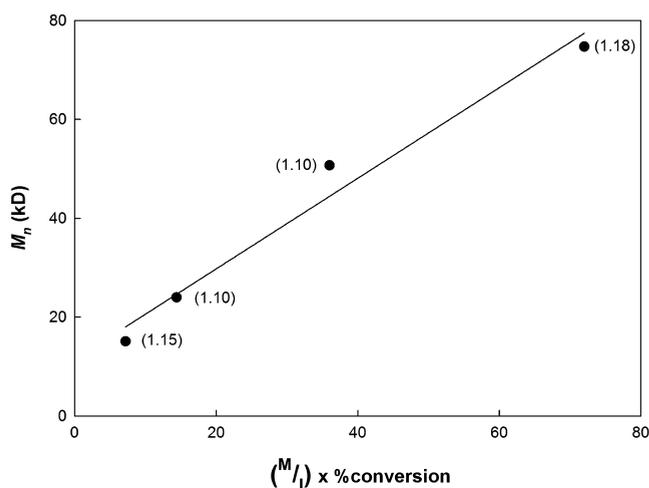
**Figure 4.** Linear relationship observed between  $M_n$  and monomer/initiator ratio of PLA produced from the ROP of L-lactide by **1b** in  $\text{CH}_2\text{Cl}_2$ . PDI values are provided in parentheses.
