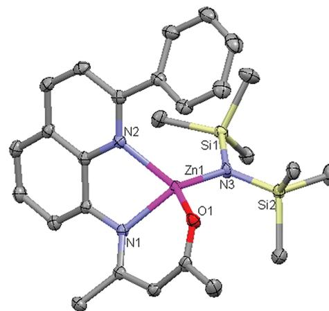
**Figure 2.** X-ray crystal structure of **4a** with thermal ellipsoids drawn at the 50% probability level. The hydrogen atoms are omitted for clarity.
