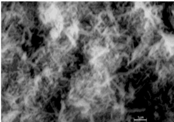
**Figure 1.** Scanning electron microscopy of ZnO nanowires.
