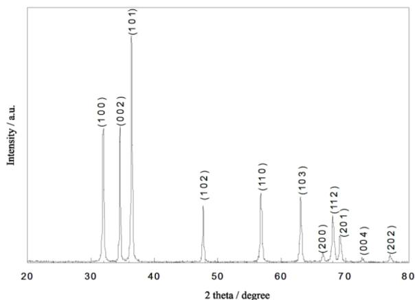
**Figure 2.** X-ray diffraction spectra of ZnO nanowires.
