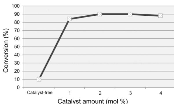
**Figure 4.** The effect of catalyst amount on synthesis of compound **3a**. Reaction time: 20 min.
