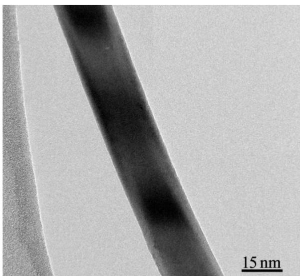
**Figure 3.** TEM image of the ZnO nanowires grown by solvothermal synthesis method.
