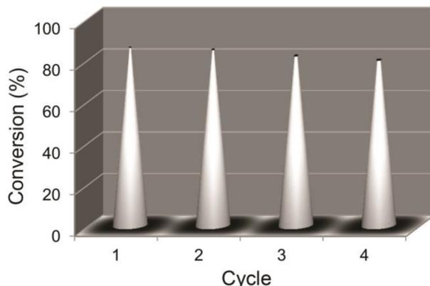
**Figure 5.** Recyclability of the catalyst. Reaction time: 20 min.
