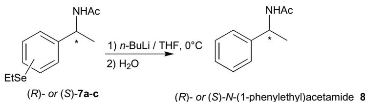
**Scheme 2.** Chemical reaction performed to transform organoselenium amides **7a–c** into (*R*)- and (*S*)-*N*-(1-phenylethyl)acetamide **8**.
