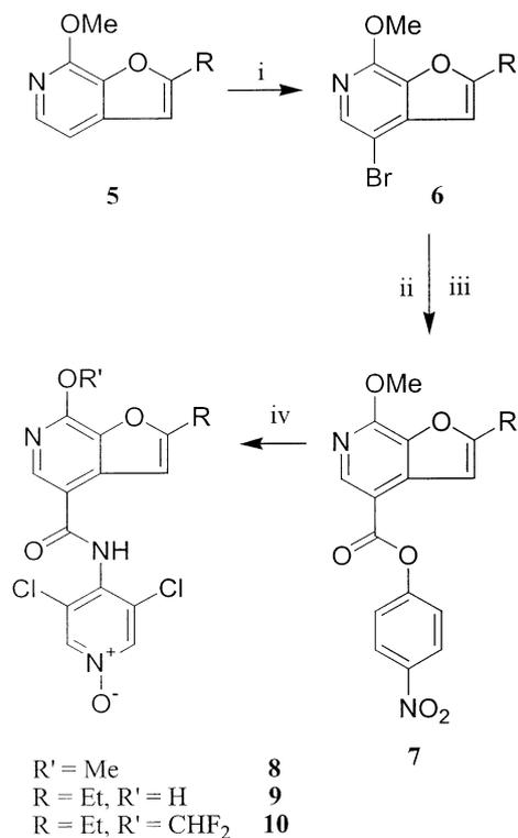
**Scheme 2.** Reagents and conditions: (i) NBS, MeCN; (ii) CO,  $\text{Pd}(\text{OAc})_2$ , bis-diphenylphosphinopropane,  $\text{NEt}_3$ , THF,  $\text{H}_2\text{O}$ ; (iii) *p*-nitrophenol, EDC·HCl, DMAP,  $\text{CH}_2\text{Cl}_2$ ; (iv) 4-amino-3,5-dichloropyridine-*N*-oxide, NaH, DMF.
