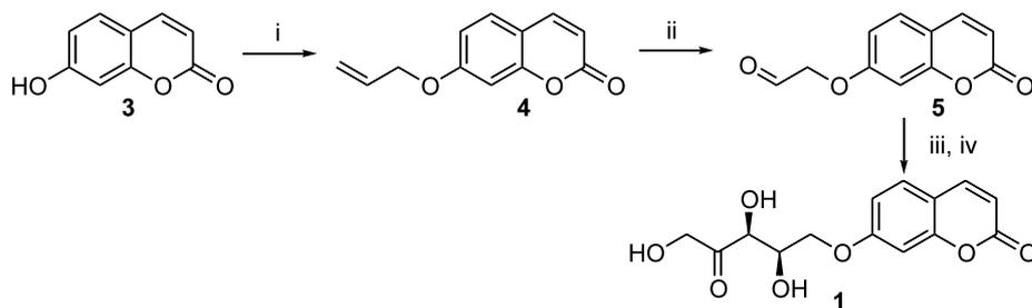
**Scheme 2.** Synthesis of the fluorogenic substrate. (i)  $\text{CH}_2=\text{CH}-\text{CH}_2\text{Br}$ ,  $\text{K}_2\text{CO}_3$ , 96%; (ii)  $\text{O}_3$ ,  $\text{Me}_2\text{S}$ , 62%; (iii) RAMA, DHAP, mCD; (iv) acid phosphatase, 35%.
