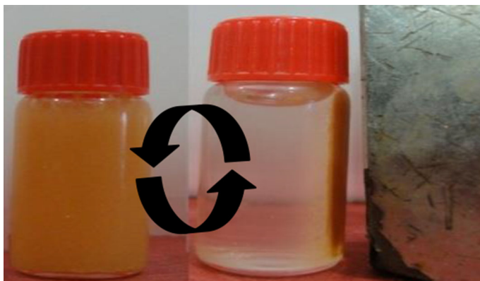
Fig. 7 Magnetic recovery of the basic nanocatalyst at the end of reactions
