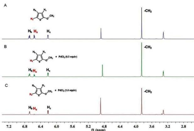
**Figure 1**  $^1\text{H}$  NMR spectra obtained in deuteromethanol ( $\text{CD}_3\text{OD}$ ). A: **1a**; B: **1a** +  $\text{PdCl}_2$  (0.5 equiv); C: **1a** +  $\text{PdCl}_2$  (1.0 equiv).
