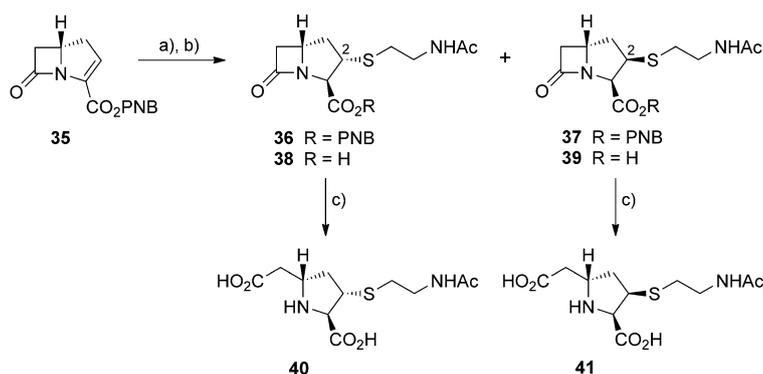
**Scheme 3.** Synthesis of 2-*N*-acetylcysteaminy-CMP diastereomers. a) *N*-acetylcysteamine, DBU, CH<sub>3</sub>CN; b) H<sub>2</sub>, 10% Pd/C, KHCO<sub>3</sub>, 2:1 THF/H<sub>2</sub>O; c) HPLC separation/lyophilization.
