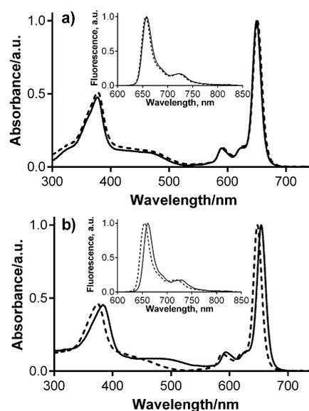
**Figure 2.** Normalized absorption and fluorescence emission (inset) spectra of studied TPyzPz in THF. a) **1Zn** (full line), **6Zn** (dashed line). b) **4Zn** (full line), **5Zn** (dashed line). Emission spectra were corrected for detector response.
