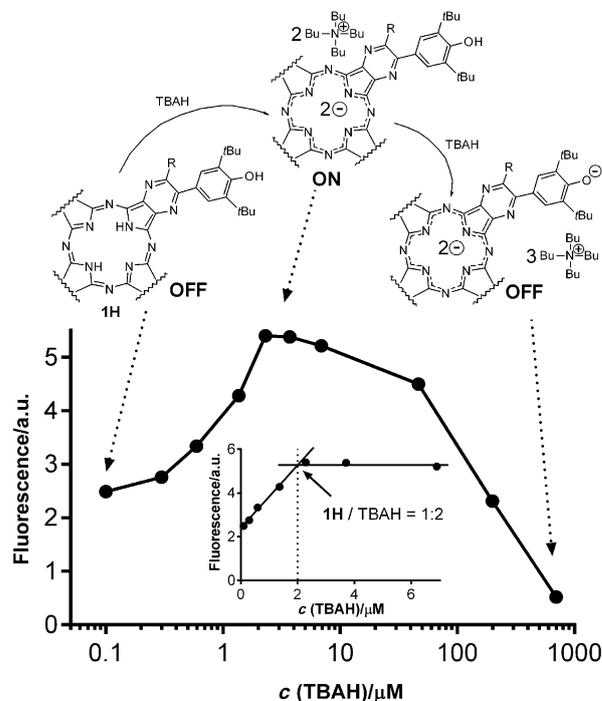
**Figure 5.** Concept of OFF-ON-OFF switching. Changes in the fluorescence of **1 H** in MeCN upon addition of TBAH;  $c(\mathbf{1 H}) = 1 \mu\text{M}$ ,  $\lambda_{\text{exc}} = 600 \text{ nm}$ ,  $\lambda_{\text{em}} = 669 \text{ nm}$ . Inset: enlarged part of the graph at lower TBAH concentrations.
