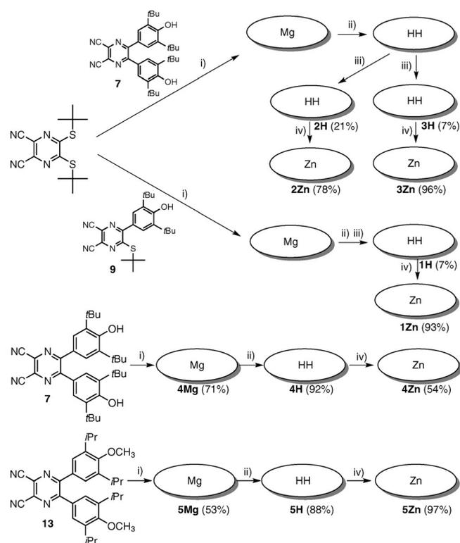
**Scheme 2.** Synthesis of TPyzPzs. i) Mg, BuOH, reflux; ii) TsOH, THF, RT; iii) separation of congeners; iv) Zn(CH<sub>3</sub>COO)<sub>2</sub>, pyridine, reflux.
