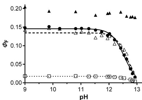
**Figure 4.** Dependence of the  $\Phi_F$  value on the pH of the buffer solution for **1 Zn** (dots, full line), **2 Zn** (open triangles, dashed line), **3 Zn** (open squares, dotted line) and **6 Zn** (full triangles) incorporated in the microemulsion. Symbols represent experimental data, and the lines are the best fit.
