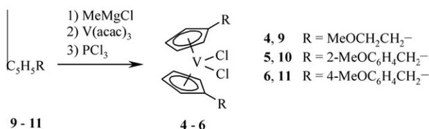
Scheme 2. Synthesis of ring-substituted vanadocene dichlorides **4–6**.
