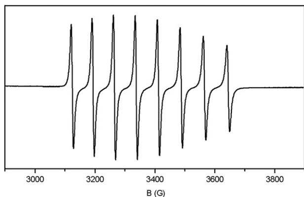
Fig. 1. EPR spectrum of dichloromethane solution of compound **4** ( $\nu = 9.428$  GHz).
