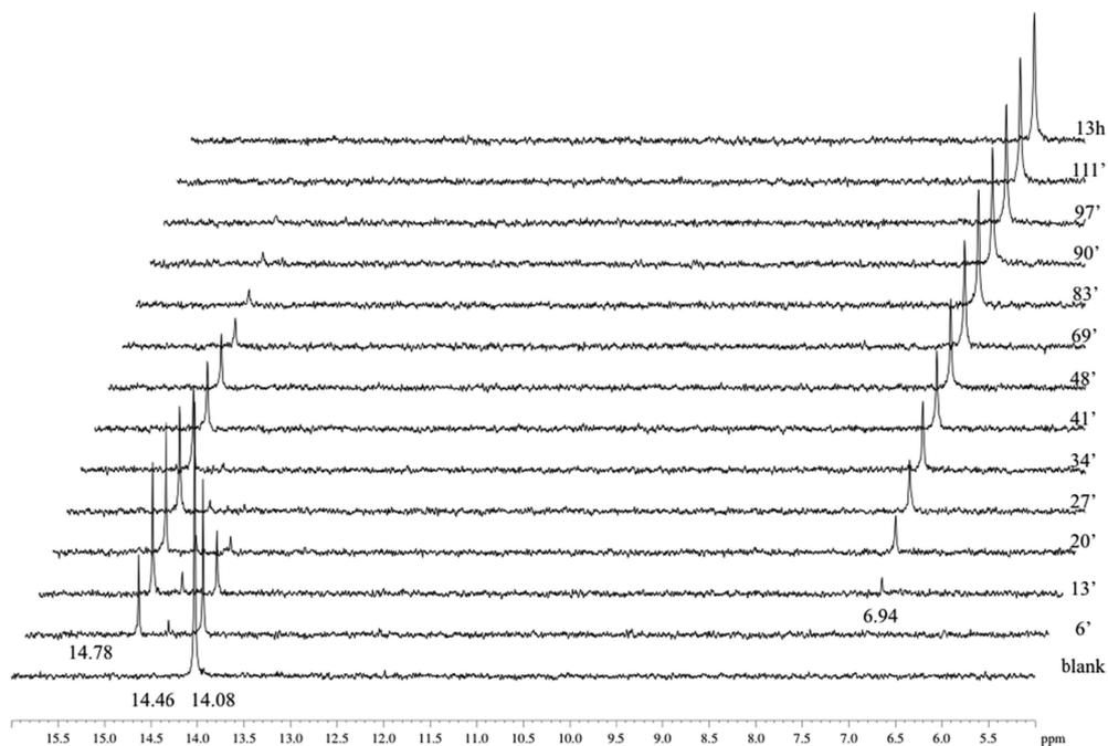
**Figure 4.**  $^{31}\text{P}$  NMR kinetic study of **21** in the presence of carboxypeptidase Y. Conditions: 5.1 mg of **21** in 200  $\mu\text{L}$  of acetone- $d_6$  + 400  $\mu\text{L}$  of Trizma buffer (pH 7.4), 0.3–0.5 mg of carboxypeptidase Y in 200  $\mu\text{L}$  of Trizma buffer (pH 7.4).
