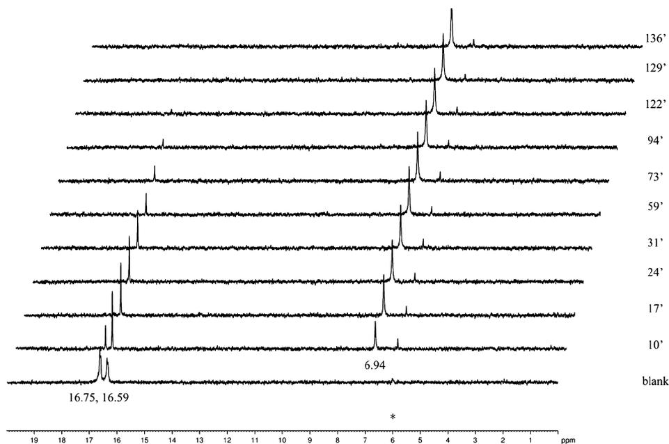
**Figure 5.**  $^{31}\text{P}$  NMR kinetic study of **65** in the presence of carboxypeptidase Y. Conditions: 4.9 mg of **65** in 200  $\mu\text{L}$  of acetone- $d_6$  + 400  $\mu\text{L}$  of Trizma buffer (pH 7.4), 0.3–0.5 mg of carboxypeptidase Y in 200  $\mu\text{L}$  of Trizma buffer (pH 7.4). \* Phosphate impurity in Trizma buffer; in blank and remains unchanged throughout.
