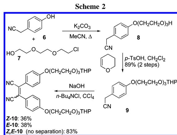
give **9**, oxidative coupling with carbon tetrachloride under basic conditions<sup>15</sup> gave a mixture of maleonitrile **Z-10** and
