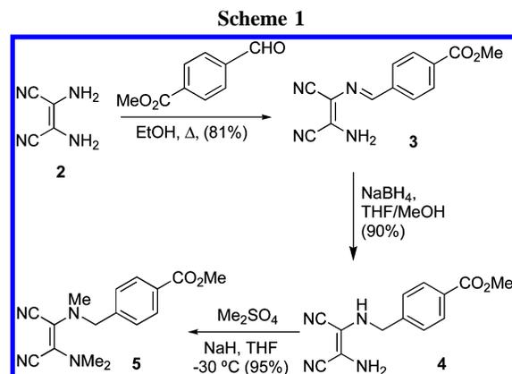
leoneitrile **2** in ethanol in the presence of methyl 4-formylbenzoate yielded the imine **3**, which was reduced with sodium borohydride in THF and methanol to give the amine **4** in 73% yield over the two steps. Subsequent methylation with dimethyl sulfate gave maleonitrile **5** in 95% yield.
