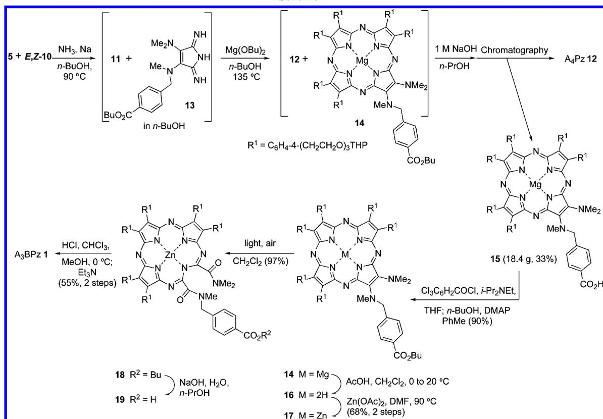
89% yield. Subsequent treatment with acetic acid yielded pure demetalated Pz **16**, which was remetalated with zinc acetate in DMF to give the zinc Pz **17** in 68% global yield. Exposure to air and light at room temperature in  $\text{CH}_2\text{Cl}_2$  gave the *seco*-Pz **18** (97%).<sup>8</sup> Finally, saponification with NaOH in *n*-propanol and acidic deprotection of the THP protecting groups gave the target Pz **1**, which could be purified on lipophilic Sephadex to give **1** (55%).
