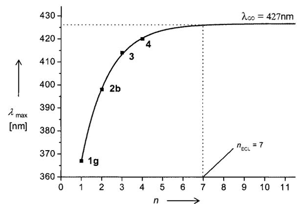
Figure 3. Long-wavelength absorption maxima of **1g**, **2b**, **3**, and **4** in  $\text{CH}_2\text{Cl}_2$ ; dependence on the number of repeat units  $n$  and the convergence to  $\lambda_\infty$  ( $n \rightarrow \infty$ )
