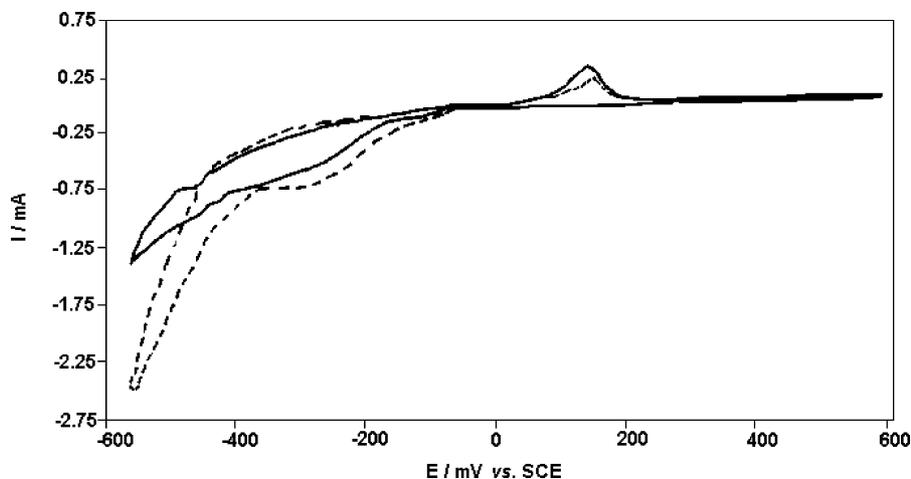
Fig. 2. CV of carbon felt disc ( $\phi = 1$  cm) in 50 mmol/dm<sup>3</sup> NiSO<sub>4</sub> at pH 3: (solid line) 1st sweep; (dashed line) 11th sweep (after reaching steady state);  $\nu = 10$  mV/s.
