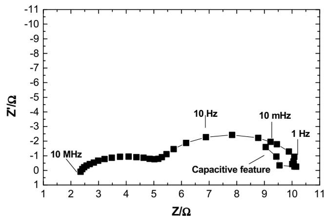
Fig. 7. Impedance plots of carbon felt ( $\phi = 1$  cm) in mmol/dm<sup>3</sup> NiCl<sub>2</sub> at -1.0 V vs. SCE.
