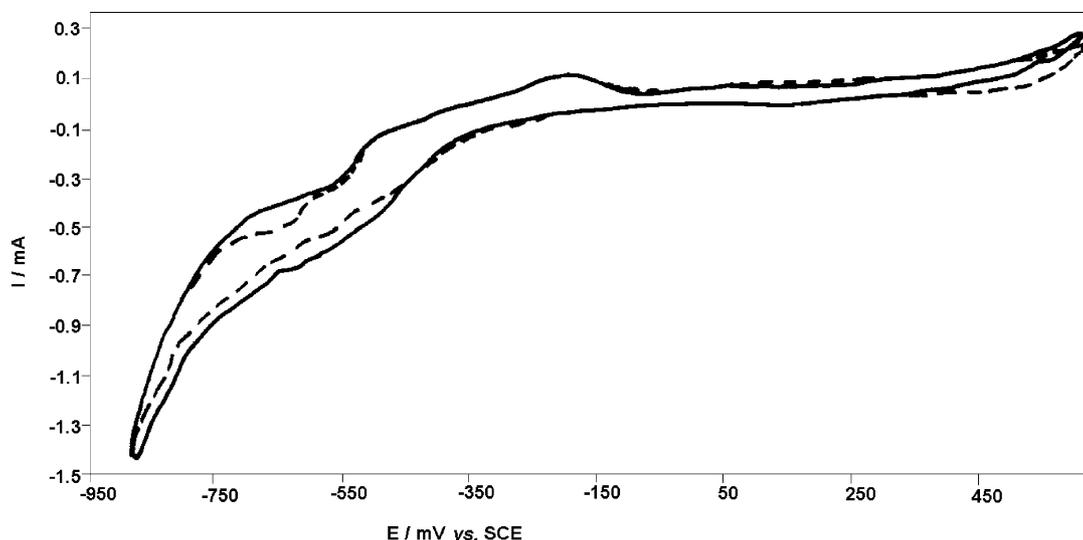
Fig. 4. CV of carbon felt disc ( $\phi = 1$  cm) in  $5 \text{ mmol/dm}^3 \text{ NiCl}_2$  at pH 3: (solid line) 1st sweep; (dashed line) 2nd sweep;  $\nu = 10 \text{ mV/s}$ .
