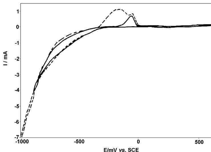
Fig. 3. CV of carbon felt disc ( $\phi = 1$  cm) in 50 mmol/dm<sup>3</sup> NiCl<sub>2</sub> at pH 3. Cathodic limit:  $-0.9$  V (solid line);  $-1.0$  V (dashed line);  $\nu = 10$  mV/s.
