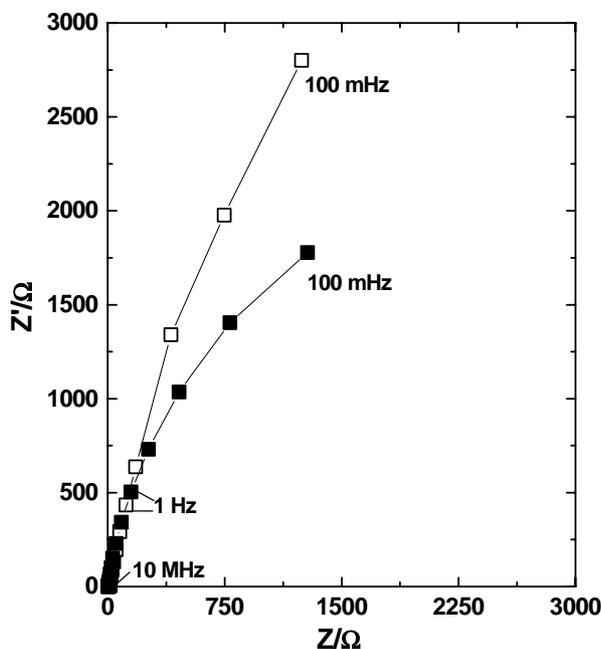
Fig. 5. Impedance plots of carbon felt disc ( $\phi = 1$  cm) in  $50 \text{ mmol/dm}^3 \text{ NiCl}_2$  (full square) and  $50 \text{ mmol/dm}^3 \text{ NiSO}_4$  (open square) at  $-0.2 \text{ V}$  vs. SCE.
