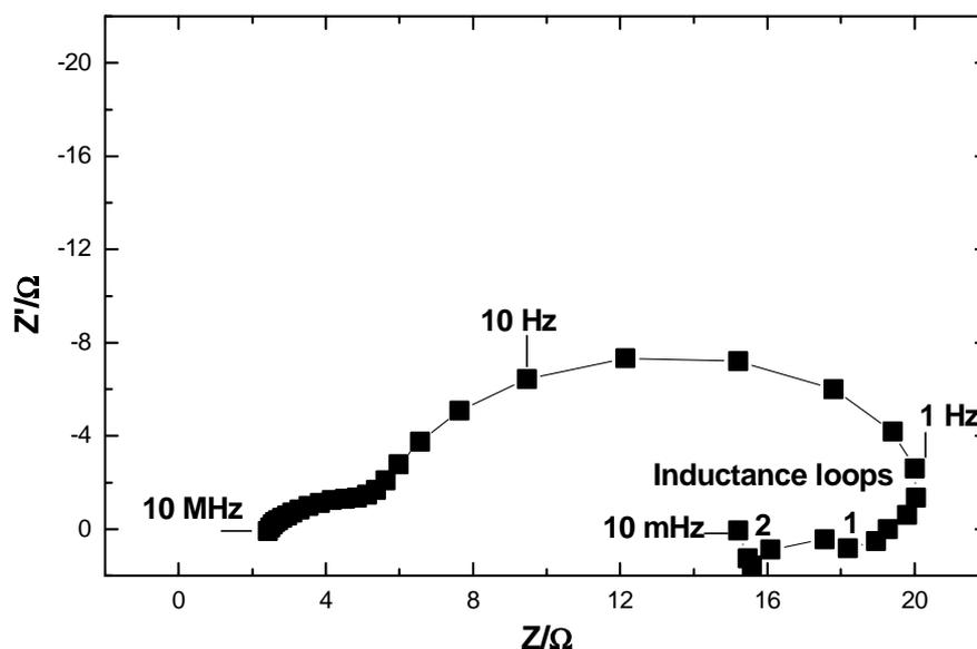
Fig. 6. Impedance plots of carbon felt ( $\phi = 1$  cm) in 50 mmol/dm<sup>3</sup> NiCl<sub>2</sub> at -0.8 V vs. SCE.
