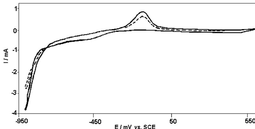
Fig. 1. CV of carbon felt disc ( $\phi = 1$  cm) in  $50 \text{ mmol/dm}^3$   $\text{NiCl}_2$  at pH 3: (solid line) 1st sweep; (dashed line) 2nd sweep;  $\nu = 10 \text{ mV/s}$ .
