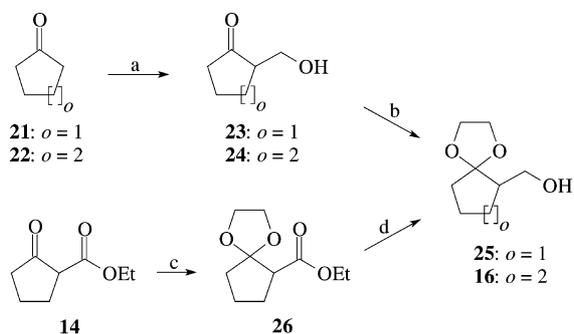
a)  $\text{CH}_2\text{O}(\text{aq})$ ,  $\text{KOH}(\text{aq})$ , 3 h 35 °C, *o* = 1: 32 %, *o* = 2: 47 %; b)  $\text{HO}(\text{CH}_2)_2\text{OH}$ , PPTS, benzene, 1 h reflux, *o* = 1: n. i., *o* = 2: 82 %, c)  $\text{HO}(\text{CH}_2)_2\text{OH}$ ,  $\text{TsOH}\cdot\text{H}_2\text{O}$ ,  $\text{CH}_2\text{Cl}_2$ , 4 d reflux, 56 %; d)  $\text{LiAlH}_4$ , THF, 3 h reflux, 73 %.
