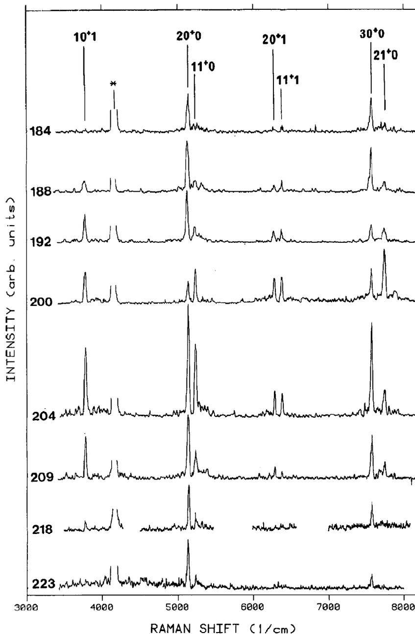
Fig. 2. The low overtone region of the resonance Raman spectra at the indicated excitation energies. Local mode labelling of the bands is used (see footnote 2). The spurious lower-order line from the Raman shifter has been removed and this region denoted with an asterisk.
