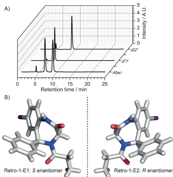
**Figure 1.** A) Chiral HPLC separation of enantiomers of Retro-1. B) Structural determination of the Retro-1 enantiomers by X-ray crystallography.
