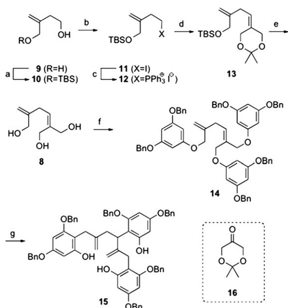
Scheme 2. Preparation of **15**: reagents and conditions; (a) TBSCl, NaH, THF, -10 °C, 43%. (b) I<sub>2</sub>, Imid., PPh<sub>3</sub>, THF, rt. (c) PPh<sub>3</sub>, CH<sub>3</sub>CN, reflux. (d) *n*-BuLi, DME, then **16**, -78 to 0 °C, 83% in three steps. (e) AcOH/H<sub>2</sub>O/THF=1:1:1, rt, 84%. (f) **7** (P=Bn), DEAD, PPh<sub>3</sub>, THF, 0 °C to rt, 50%. (g) Me<sub>3</sub>Al, CH<sub>2</sub>Cl<sub>2</sub>, 0 °C to rt, 84%.
