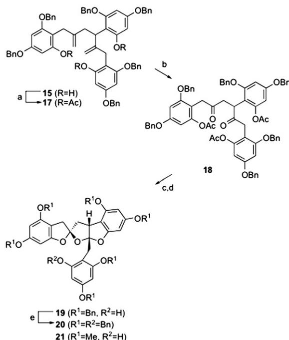
Scheme 3. Preparation of spiro[furan-furofuran] **20**: reagents and conditions; (a) Ac<sub>2</sub>O, NaH, THF, 0 °C, 92%. (b) O<sub>3</sub>, CH<sub>2</sub>Cl<sub>2</sub>, -78 °C, then PPh<sub>3</sub>, 83%. (c) K<sub>2</sub>CO<sub>3</sub>, MeOH, 0 °C. (d) TsOH, CH<sub>2</sub>Cl<sub>2</sub>, 0 °C to rt, 81% in two steps. (e) BnBr, NaH, DMF, 0 °C, 97%.
