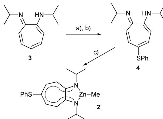
**Scheme 2** Reagents and conditions: (a) Br<sub>2</sub>, CH<sub>2</sub>Cl<sub>2</sub>, 0 °C to RT, 1 h, 90%; (b) PhSH, K<sub>2</sub>CO<sub>3</sub>, DMF, 70 °C, 16 h, 99%; (c) ZnMe<sub>2</sub> (1.7 eq.), toluene, RT, 3 h, 88%.
