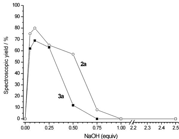
Figure 6. Profiles of the reaction between ethyl nitroacetate (**1a**) and allyl alcohol (open circles) or styrene (solid squares). The data shows the calculated yield after 18 h depending on the amount of sodium hydroxide used in the reaction.
