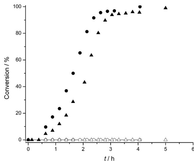
Figure 5. Condensation reaction of methyl nitroacetate (**1b**) with 3-buten-1-ol (circles) and 4-penten-1-ol (triangles) catalysed by DABCO at 60°C. Effect of solvent on the conversion of the dipolarophiles to the cycloadducts **4b** and **5b**, respectively. Heavy water (solid markers) deuteriochloroform (open markers).
