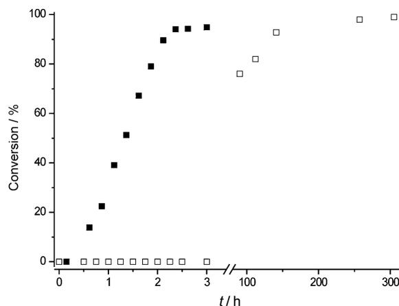
Figure 4. Condensation reaction of methyl nitroacetate (**1b**) with allyl alcohol catalysed by DABCO at 60°C. Effect of solvent on the conversion of dipolarophile to cycloadduct **2b**. Heavy water (solid squares); deuteriochloroform (open squares).<sup>[41]</sup>
