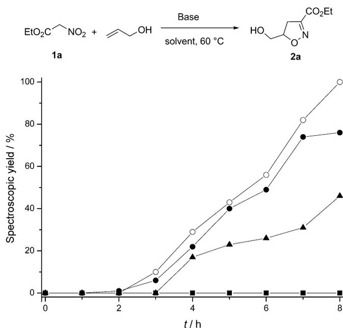
Figure 1. Reaction profiles for the condensation reaction of ethyl nitroacetate (**1a**) and allyl alcohol in water or chloroform as solvent or neat. Reaction in water with extraction in chloroform (solid circles); reaction in water followed by concentration (open circles); reaction in chloroform (solid squares) and neat (solid triangles).
